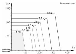
The KR 6 R700 CR is designed for a rated payload of 3 kg in order to optimize the dynamic performance of the robot. With reduced load center distances, higher loads up to the maximum payload may be used. The specific load case must be verified using KUKA.Load. For further consultation, please contact KUKA Support.
